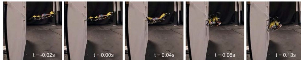
Fig. 14. Sequential images from a video footage showing the mid-flight collision when the robot had the translational speed of 1.5 \text{ m.s}^{-1} . The images reveal that the impact triggered the folding of all arms in less than 0.15 s.
